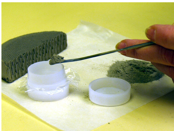
Materials are pulverized to a maximum 250µm and loaded in XRF sample cups or sample bags for analysis.
